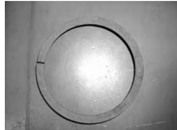
No color or ID groove around surface
