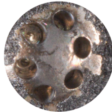
Injector after one P.i. treatment.
