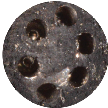
Injector before P.i. treatment.
