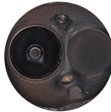
Cylinder head before P.i. treatment.
