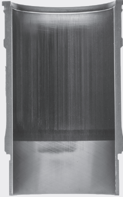
Severely Scuffed Liner
