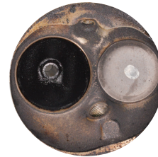
Cylinder head after one P.i. treatment.
